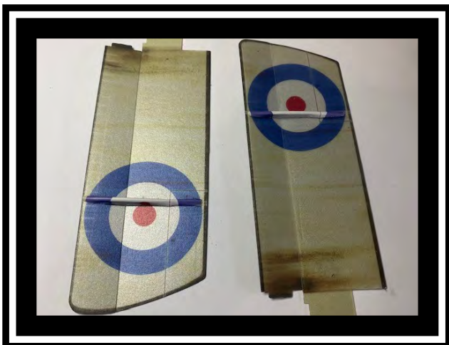
Half of lower wing with "rib" in place. This gives some curvature to top and bottom wings.
