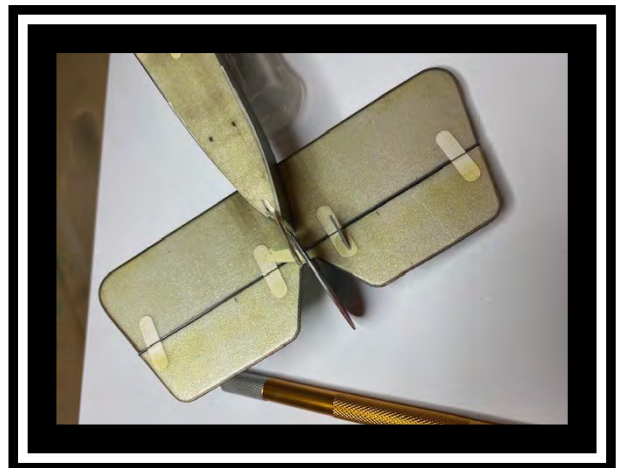
Rudder and elevator hinged and control horns in place.
