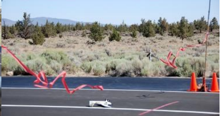
LANDING GEAR SNAGGED RIBBON, PLANE FLIPPED AS RIBBON BROKE, AND SETTLED ON RUNWAY INVERTED
