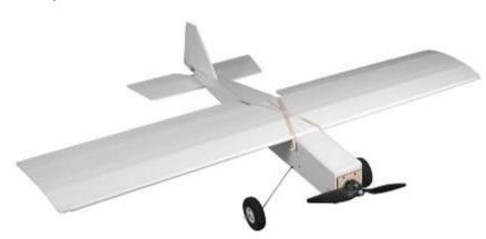
it is made with their white foamboard they call Maker Foam. As a result, you can install lights on the inside of the plane and they will show up quite well. I also installed external LEDs under the leading edge, Red for left wing and Green for right wing. You can find various
