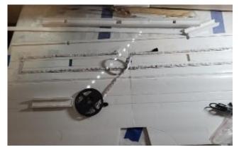
In the wing, I simply taped the LED strips around the internal wing spar and brought the leads out of the hole where the aileron leads exit into the fuselage. This pic shows the wing laid open before it is hot glued together. I don't know why there is a line of white dots in this picture; apparently, the LEDs reflected the flash.
