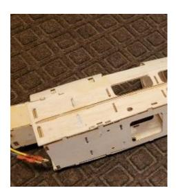
Backing up to that "Paste" picture, I'll share something I learned that led me to believe I wouldn't be turning out a museum piece. This plywood doubler A1-3 is "pasted" to the front portion of each balsa fuselage side. I applied some good ol' Titebond to join the accurately-cut doublers on each side of the fuselage, and after ensuring they were just perfect, I laid some weight on them to make sure everything was good to go.
