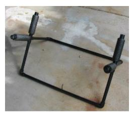
Assemble as shown in the picture. I didn't glue any of the parts. They fit very tightly and the stand can be easily broken down into pieces to save space. Jim
