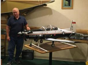
Bob Ingram brought in his recently completed ESM T-6 Texan II. It has an 80" wingspan and has a DLE35RA gasoline engine. The plane weighs in at about 18 lbs. And only required a few ounces of weight in the tail to balance. Rick Burgess was the primary builder teaching Bob about building BIG plane with fiberglass fuselages. Bob hopes to fly the model soon. UPDATE: Actual maiden flight was by Tom Rainwater on Tuesday May 3rd. Bob flew it for the 2nd flight later in the day. Beautiful plane.
