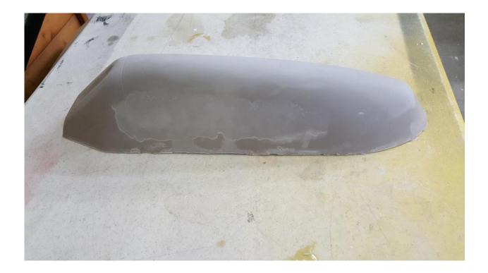
So after the cement set up it popped right out of the canopy without any problems resulting in a pretty smooth plug to work with. This plug will need to be sanded and filled in some areas before it can be used for pulling a replacement canopy. In order to get a "good" plastic canopy you need a "perfect" plug. Any imperfections in the plug will transfer to your canopy.
