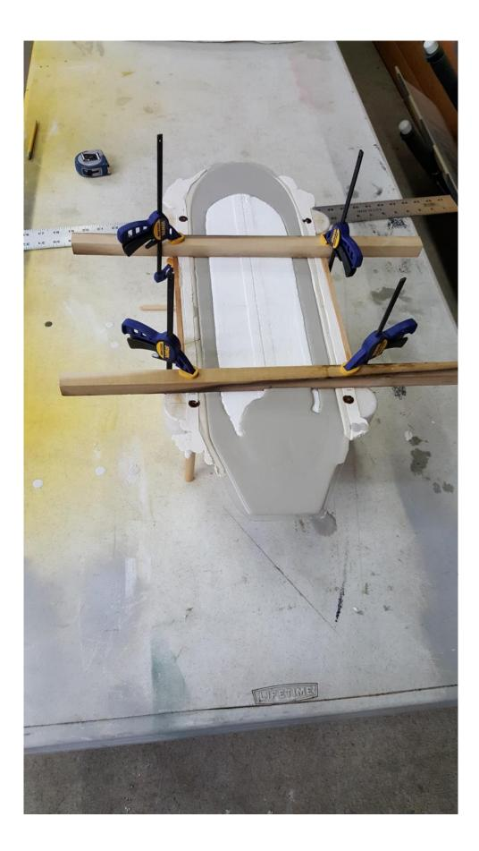
Next I mixed up the UltraCal-30 casting cement and poured in directly into the canopy. I did not use any release agent on the canopy. A previous attempt using PAM cooking oil left a rough finish on the final plug.
