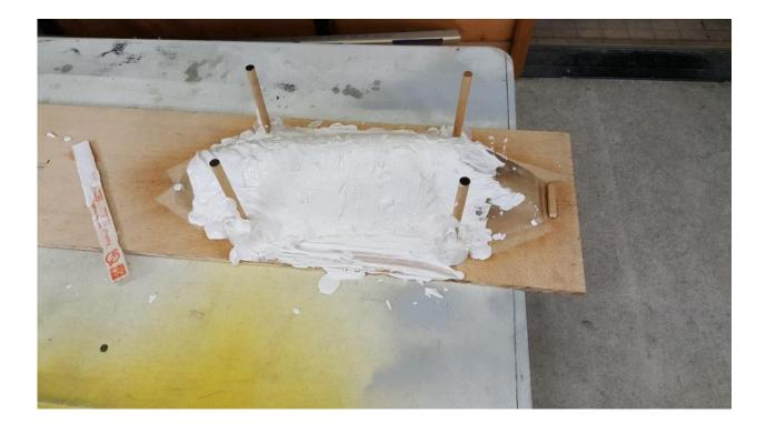
Next I applied a liberal amount of Hydro-Cal casting cement to the outside of the canopy. I didn't need to cover it all as this material would only form a saddle to hold the canopy shape and hold the opening level so I can pour liquid casting cement on the inside of the canopy.
