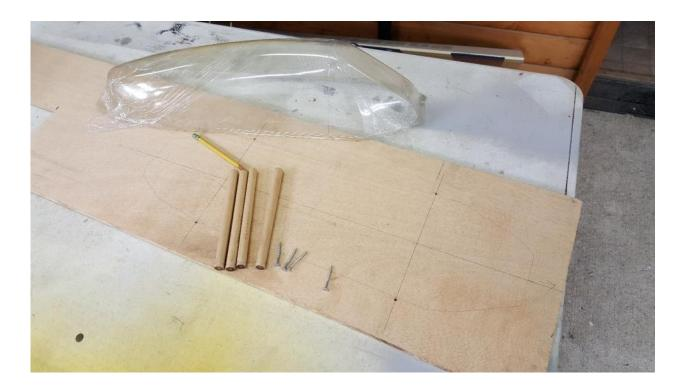
I placed the canopy on a piece of plywood and drew the outline of the canopy. I then drilled holes just outside the canopy outline to secure dowel legs to the board with screws from the bottom. These legs not only held the canopy down but also prevent the canopy from flexing outward.
