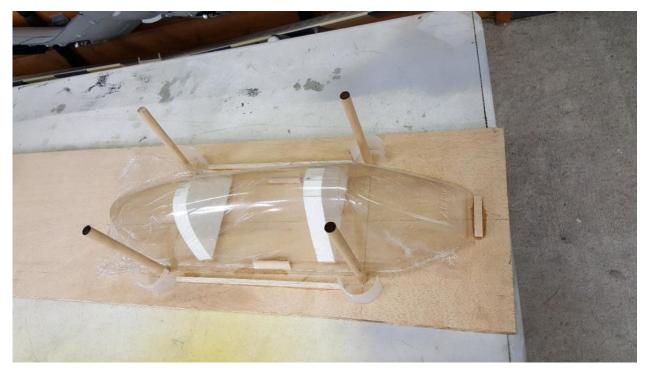
After attaching the legs I added supports inside the canopy to prevent it from flexing in, I cut two spray can lids in half to provide a dam to hold more cement around the legs supports. I also cut two foam bulkheads to help the canopy maintain its shape while applying the casting cement to the outside of the canopy.
