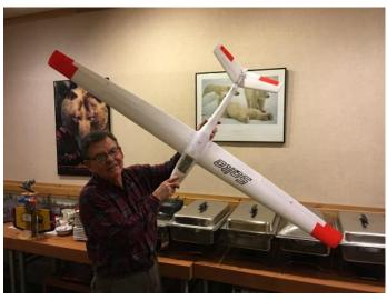
Bill Hand brought in a very unique Salto glider from ST Models. The glider uses EDF propulsion that retracts back into the fuselage when not needed to reduce drag. With the top mounted EDF unit and the installation of wheels on the fuselage you can take this aircraft off from the ground. With a 3S battery and a 71"+ wingspan this bird should fly for quite a while. Yet another beautiful glider from the Hand hanger.
