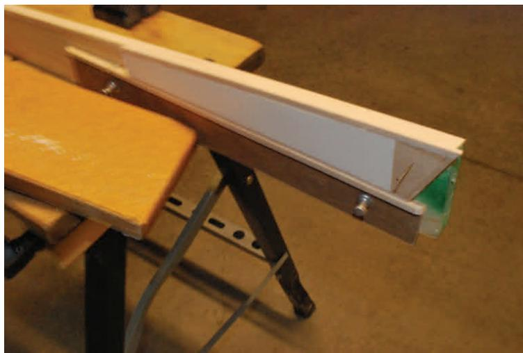
The actual process is to mount the control surface so the center line of the leading edge is lined up with the jig as shown in this second diagram from Dave's article.
