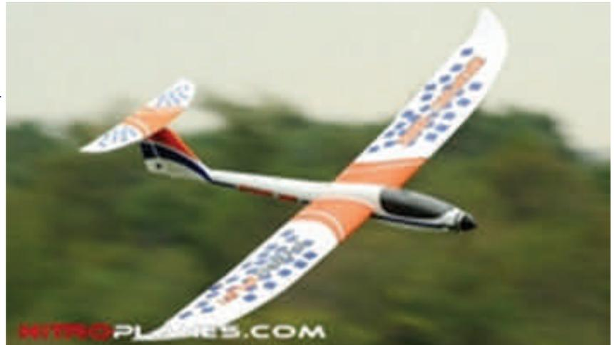
This is a large, nice easy flying plane that with a little practice will soar for an hour or more. The recommended battery is a 7.4V 1800. Power is quite adequate, and for a foamy, the quality of the plane is pretty good. It is a 4 channel plane with an easy to program ESC (you will want to activate the motor brake on this one). It comes with all electrics installed. Just add your receiver and battery. Our fearless leader maiden mine, and liked it enough to order one for himself
