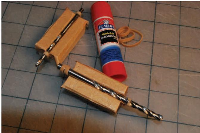
The last step is to use the finish size drill bit, 1/8" or 3/16" to hold the sandpaper in place. I have quite a collection of old sandpaper scraps and generally make these using about 120 grit. Coat the block including the groove and the paper with a glue stick and then use the drill bit and rubber bands as shown to hold it in place. Trim off the excess paper when dry and you have a nice sanding aid. Making several at once is even quicker.
