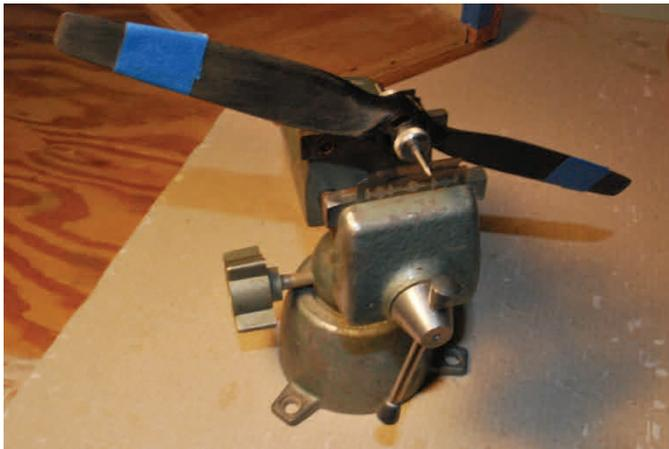
On the internet I found some plans for a home built prop balancer. It's built out of  $\frac{1}{2}$ " x 2- $\frac{1}{2}$ " poplar from Home Depot. The magnets are  $\frac{1}{2}$ " super-strong magnets from Michael's Craft Store. Originally designed for smaller electric props, the  $\frac{1}{2}$ " magnets work fine but for bigger props I would increase the magnet size up to  $\frac{3}{4}$ ". You will also need a Dubro or similar thumb balancer.
