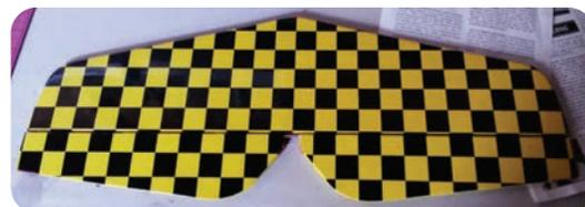
Top and Bottom of the horizontal stab and elevator
