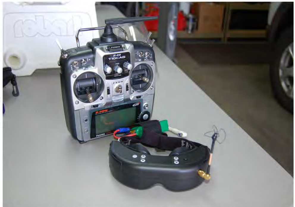
Futaba 10 c w/Fat Shark Dominator Goggles with, battery, receiver & head tracking module.
