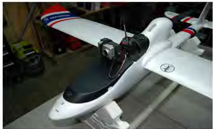
The Penguin, complete with transmitter, pan/tilt module & Go Pro
